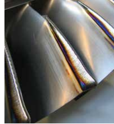
Left: Induction-assisted additive manufacturing of a component. Right: Laser cladding is a well established technology for the repair of turbine blades.
