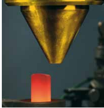
Left: Induction-assisted additive manufacturing of a component. Right: Laser cladding is a well established technology for the repair of turbine blades.
